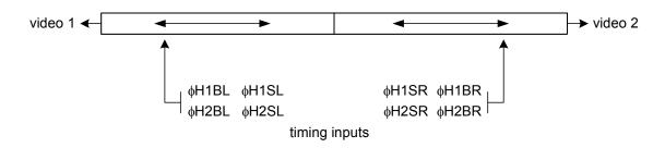
The horizontal CCD is arranged to allow the entire image to be read out of either video 1 or video 2 (mirror image). For faster read out both video 1 and video 2 may be used simultaneously. The horizontal shift register is designed as a reversible pseudo 2-phase CCD. The direction of charge transfer in the horizontal CCD is controlled by the wiring connections.
